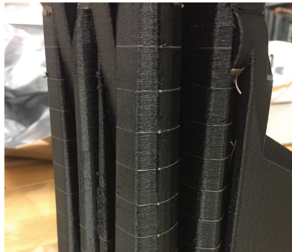
Figure 5: A FDM Nylon 12CF part printed with sparse supports, using model as support where possible and two layers of perforation with a 0.5-inch interval.
