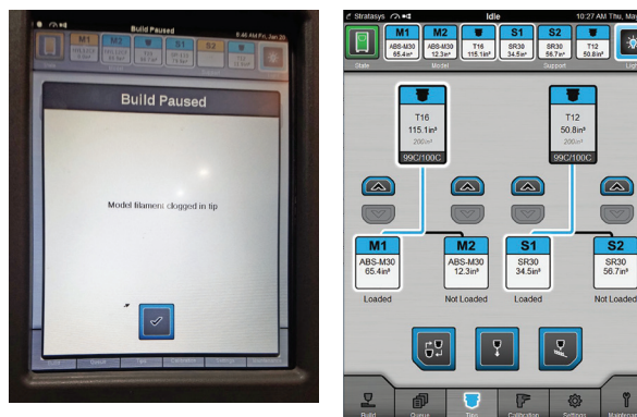
Figure 9: When printing with FDM Nylon 12CF material the build pause warning “Model filament clogged in tip” should be resolved using the procedure in Section 2.2.1 of this document.
