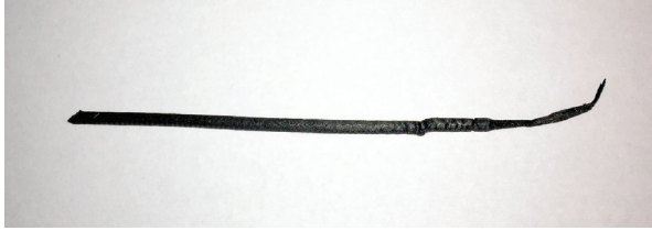
Figure 14: A section of filament that shows a kink that can correspond with the build pause warning “Model filament is clogged in tip.”
